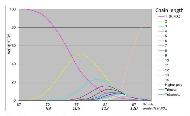
**Figure 14** Polyphosphoric acid chain length varies as a function of the P<sub>2</sub>O<sub>5</sub> content (% mass) and the grade number (% H<sub>3</sub>PO<sub>4</sub> by mass in solution), on the x-axis. Longer chain length implies more interlinked HPO<sub>3</sub> units with PO<sub>3</sub>H<sub>2</sub> end groups. The chain length increases when the solution contains less water.
