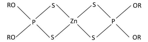
**Figure 30** Zinc dialkyl dithiophosphate (ZDDP) molecule. The bond structure around the Zn atom is indicative, it retains part of its 2+ charge and the two dithiophosphate units some of their negative charge. R denotes an organic group such as ethyl.
