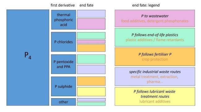
**Figure 43** Main environmental fates of true P<sub>4</sub> derivatives
